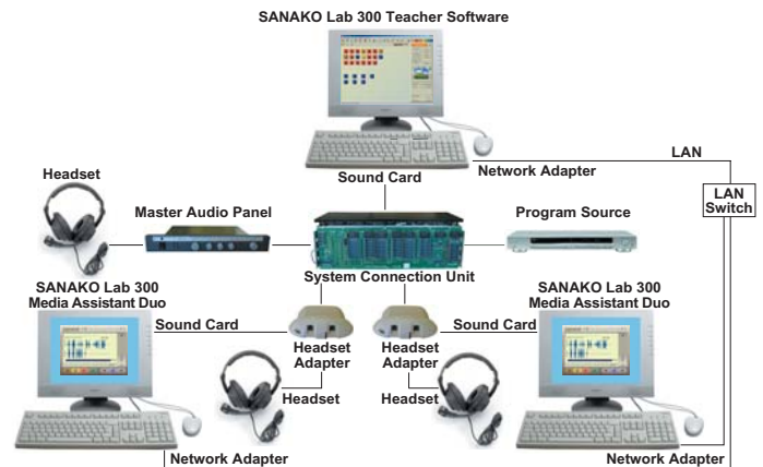
SANAKO Lab 300 system architecture
